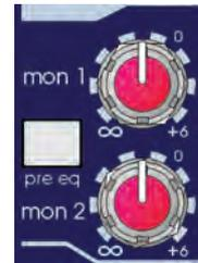
Monitor section of the dual stereo input channels
