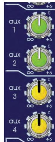
Aux sections of the dual stereo input channels
